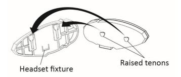
3-3-1.3 Remove the headset: Push the headset upwards to remove the headset from the fixture.
