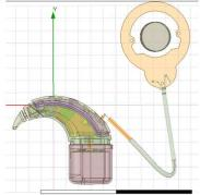
A simulation of the chip antenna ANT3216LL00R2400A was performed with a 3D model of CP1110 Sound processor in Ansys HFSS.
