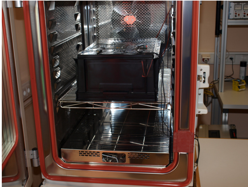
Picture 1-5: Carrier frequency stability test setup
