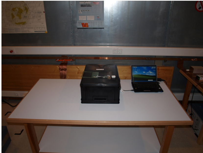
Picture 1-3: Conducted emission test setup
