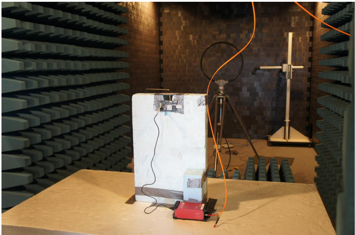
Picture 4: test setup radiated emission test 9 kHz - 30 MHz
