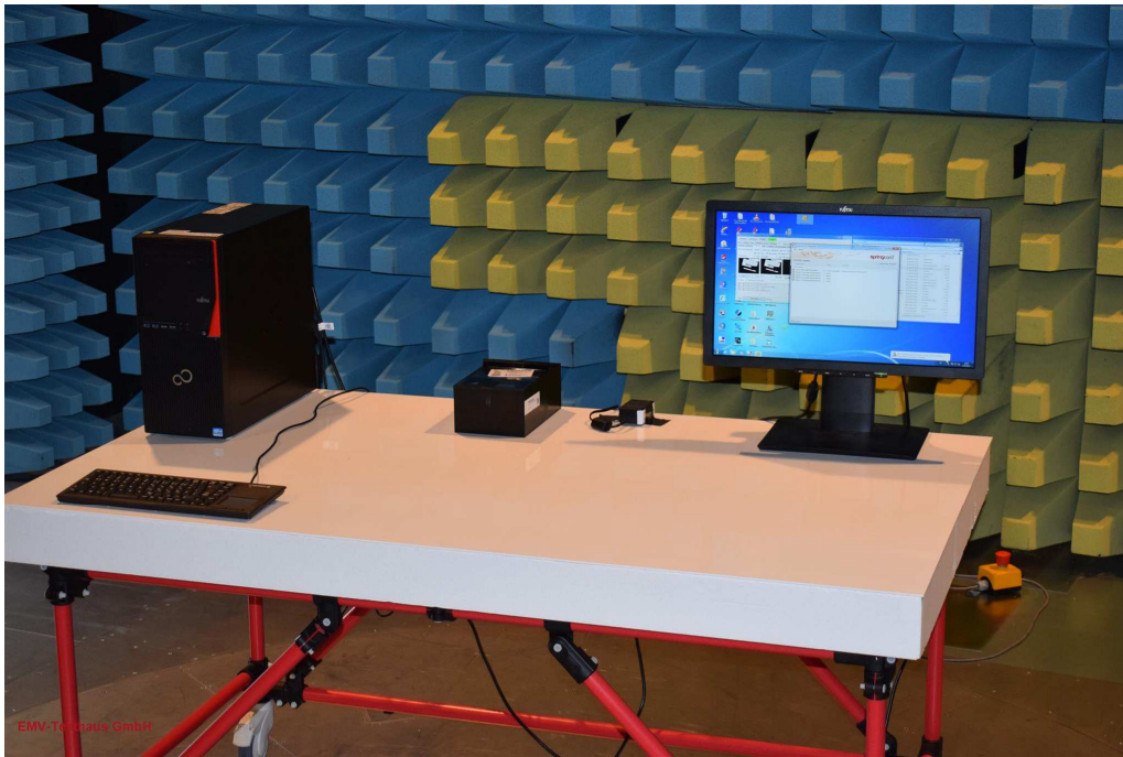
Picture 5: EUT test setup radiated emission test > 1 GHz (front view)
