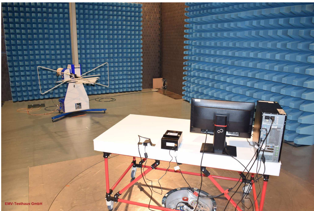
Picture 4: EUT test setup radiated emission test - 30 MHz - 1 GHz (rear view)
