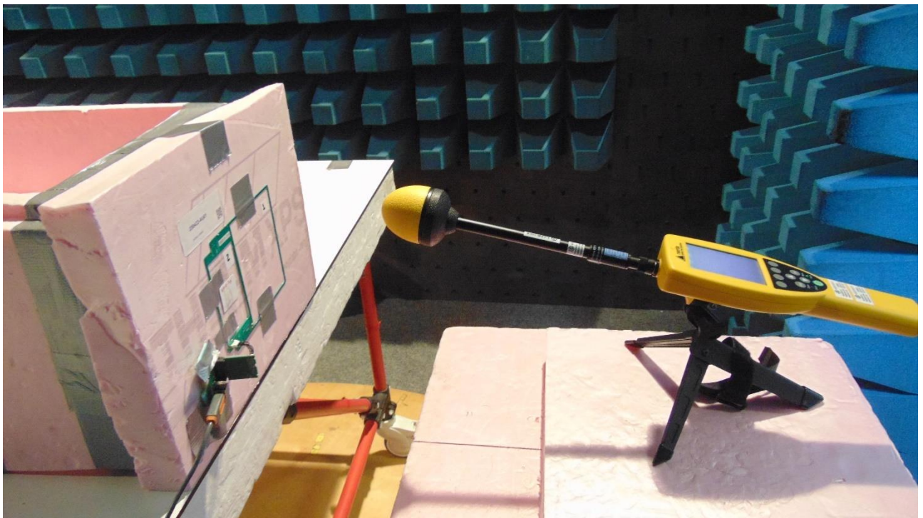
Picture 12: Setup of electric field test at a measurement distance of 20 cm, with RFID tag in Position 2
