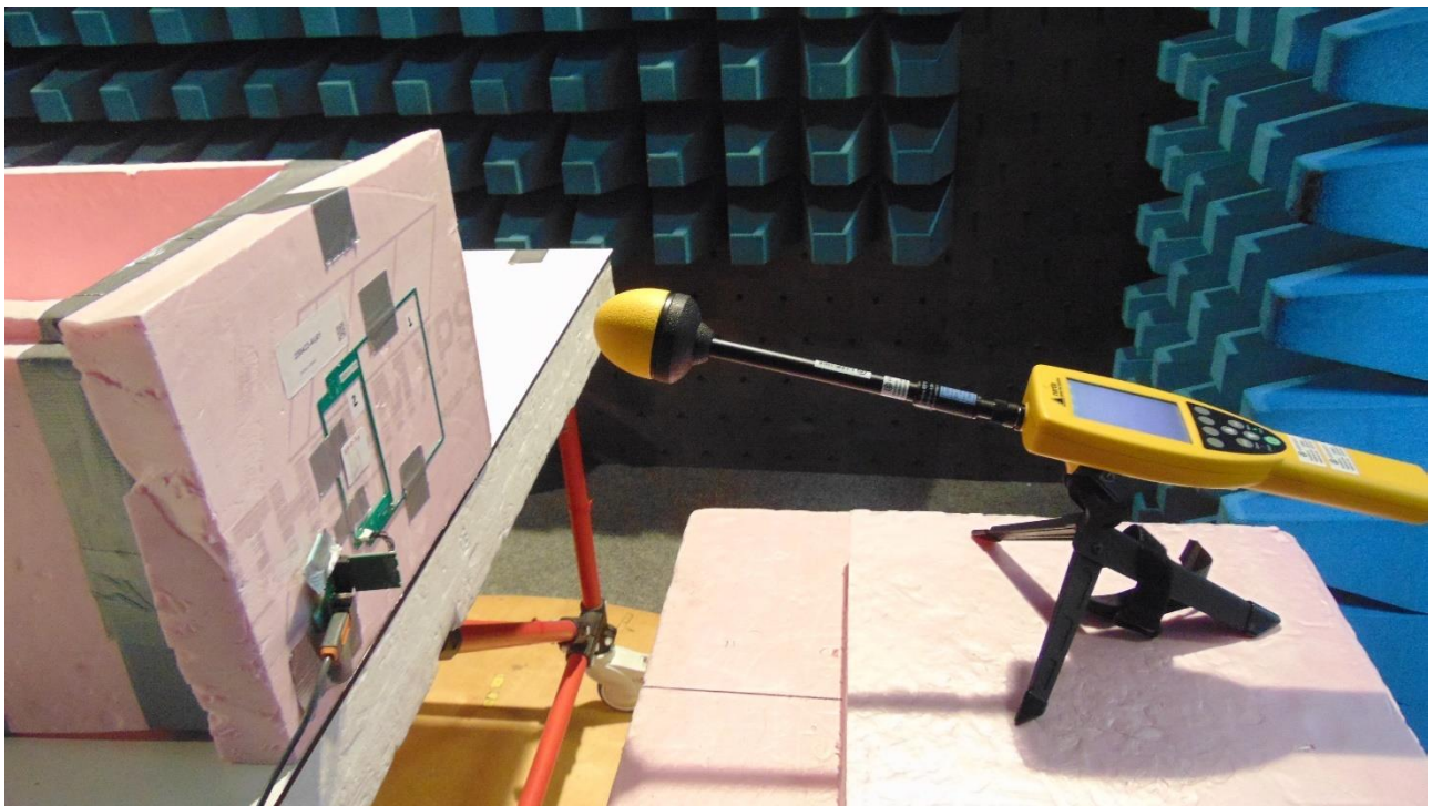
Picture 6: Setup of electric field test at a measurement distance of 20 cm, with RFID tag in Position 2
