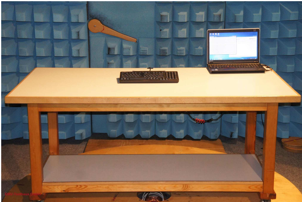
Picture 1: EUT test setup radiated emission test < 30 MHz (front view)
