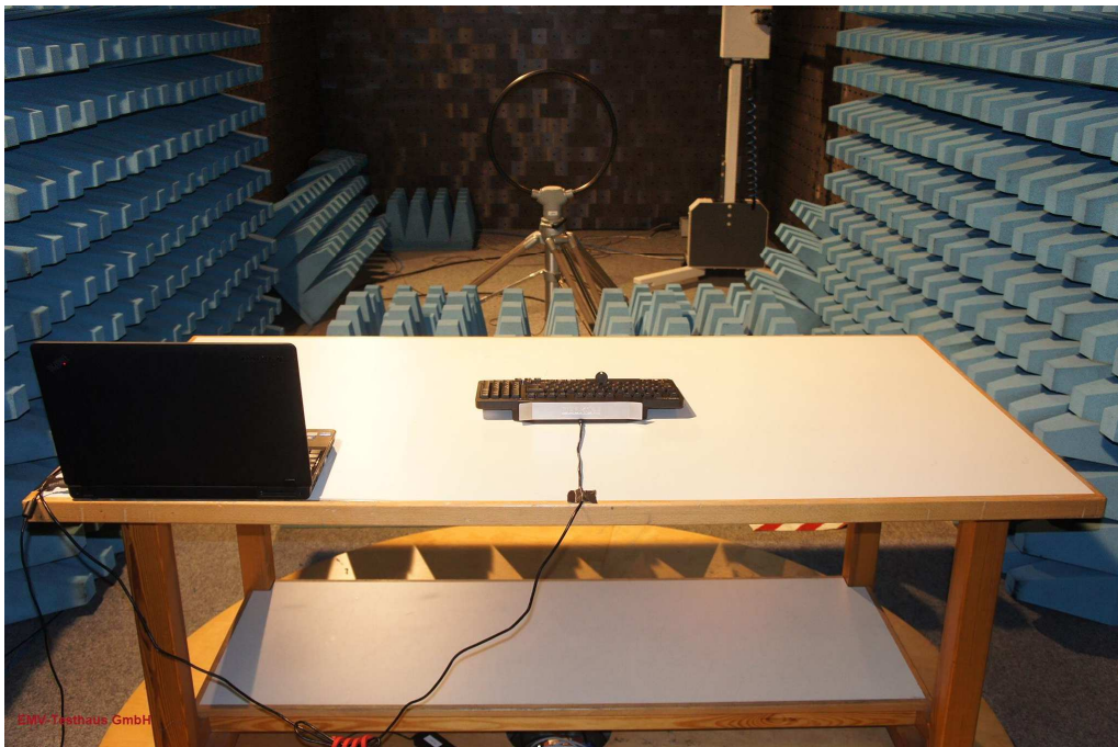
Picture 2: EUT test setup radiated emission test < 30 MHz (rear view)
