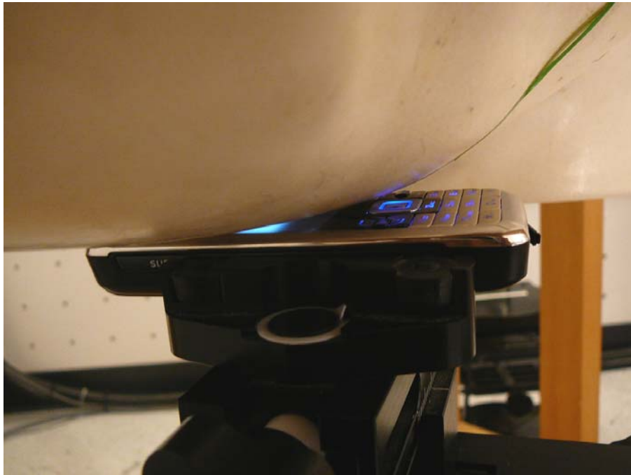
EUT Right Head Touch Setup Photo
