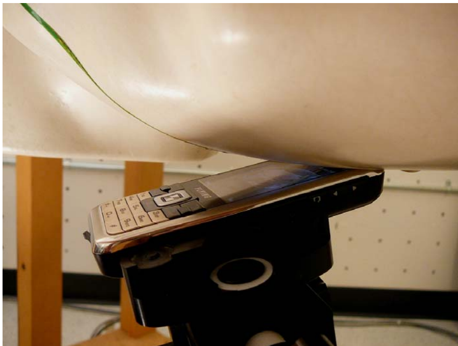
EUT Left Head Tilt Setup Photo
