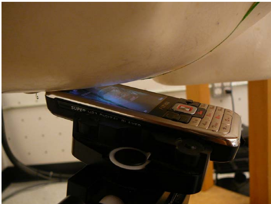
EUT Right Head Tilt Setup Photo
