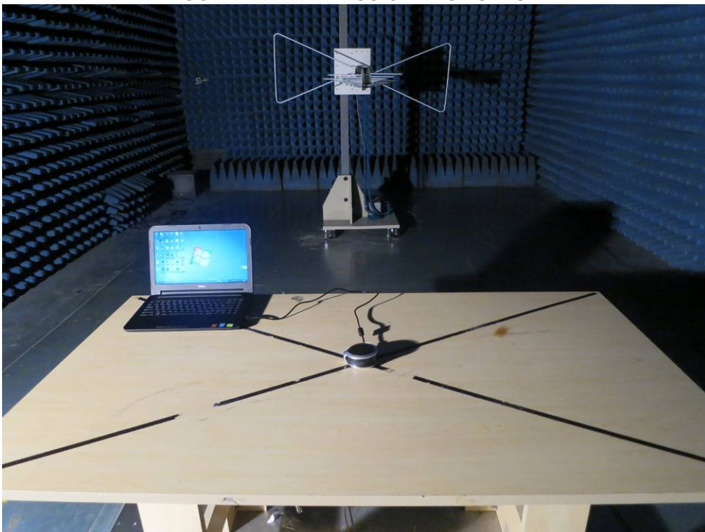
FCC RADIATED EMISSION TEST SETUP
