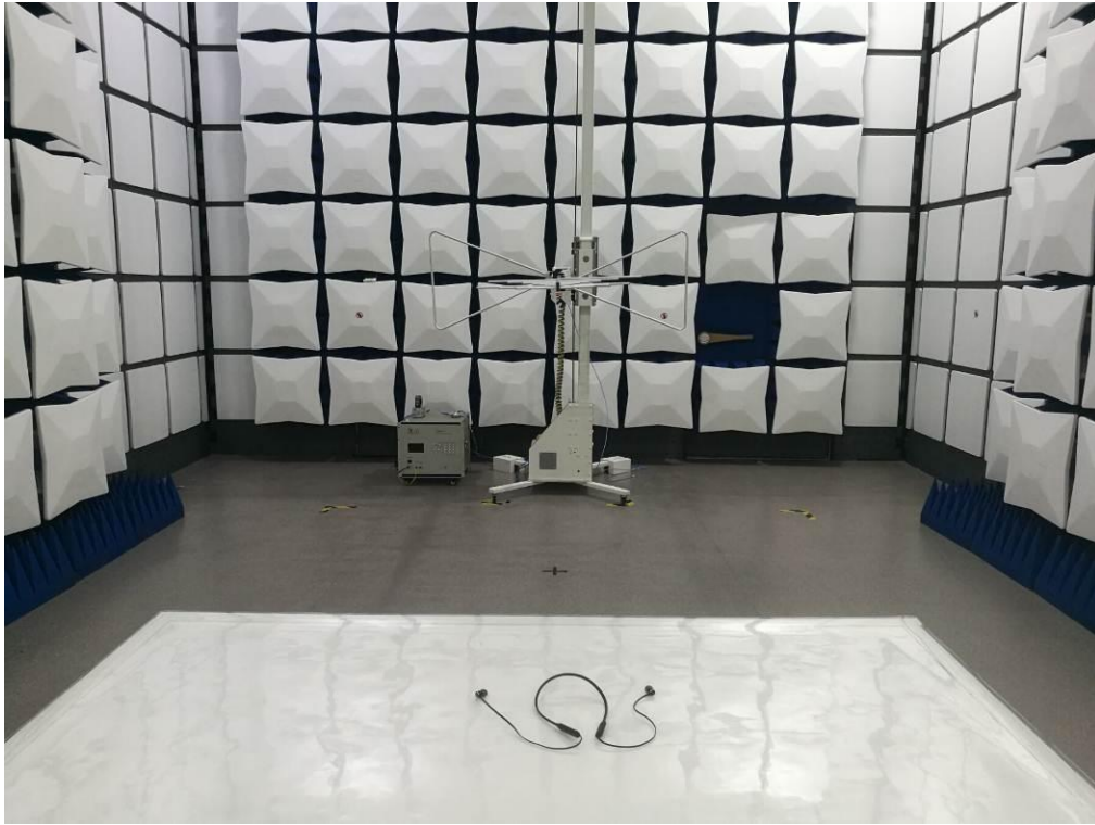
FCC RADIATED EMISSION TEST SETUP
