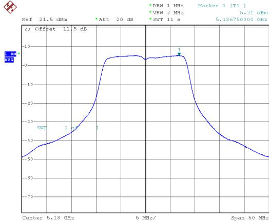
Modulation Standard: 802.11ac, VHT20 (6.5Mbps)
