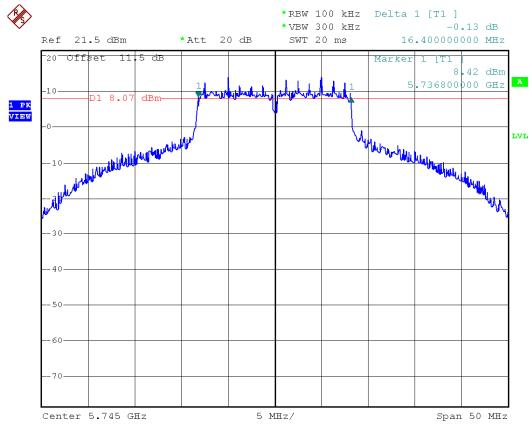
Modulation Standard: 802.11ac, VHT20 (6.5Mbps)
