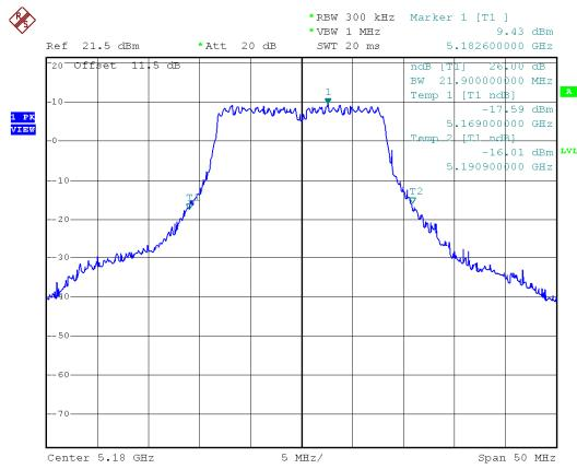
Modulation Standard: 802.11ac, VHT20 (6.5Mbps)
