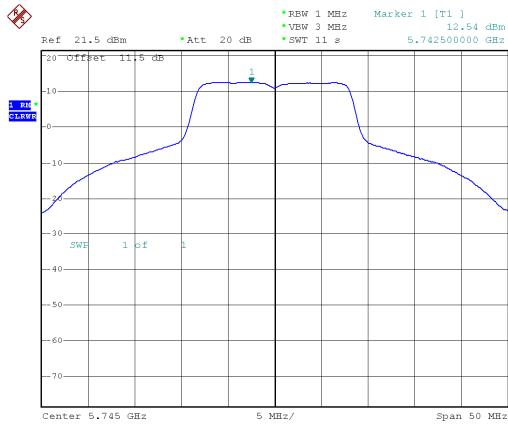
Modulation Standard: 802.11ac, VHT20 (6.5Mbps)
