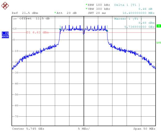
Modulation Standard: 802.11ac, VHT20 (6.5Mbps)
