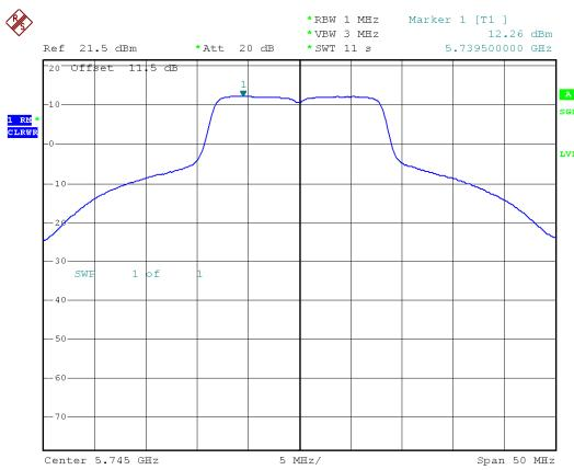
Modulation Standard: 802.11ac, VHT20 (6.5Mbps)
