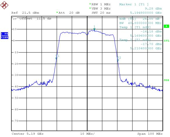
Modulation Standard: 802.11ac VHT80 (29.3Mbps)
