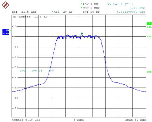
Modulation Standard: 802.11ac VHT20 (6.5Mbps)
