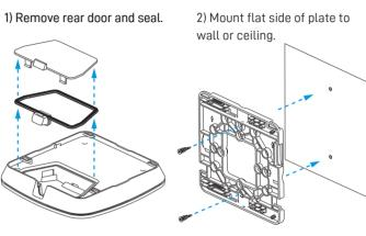
3) Connect ethernet cable to device (Port 1).
