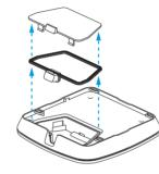
3) Place ethernet cable through seal and connect to device (Port 1). Reinstall seal and back cover. 4) Slide device down plate to lock in place.
