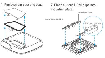
Use the adjustable rail clips to tighten to the ceiling T-Rail until secure.
