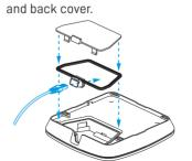
2) Secure flat side of mount to outdoor fixture. Arrows on plate pointing upwards.
