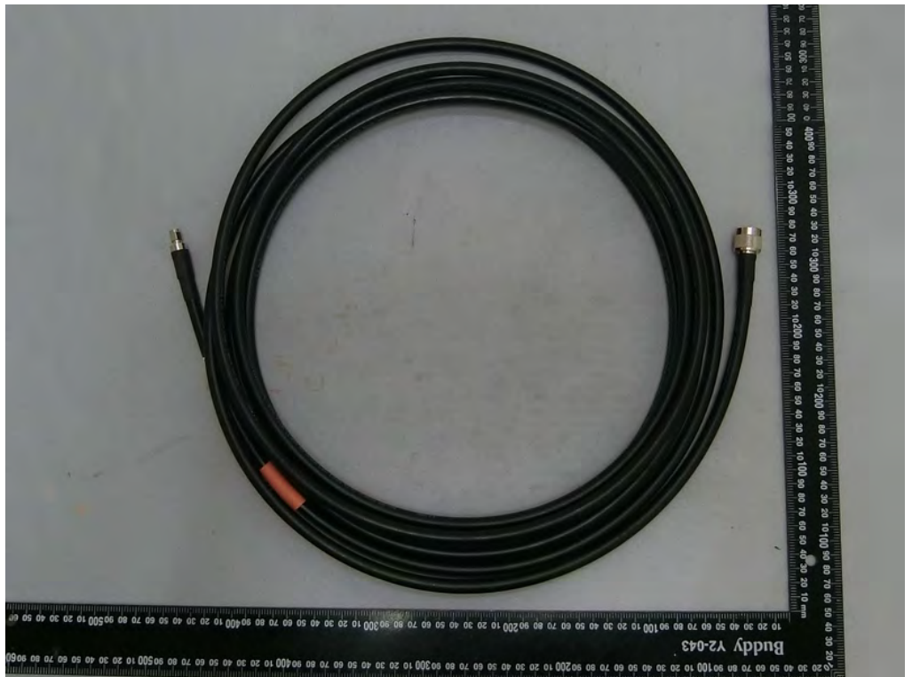
Cradlepoint to External Antenna Cable (Only for EUT 2 with WWAN ant. set 2, and 3 use)
