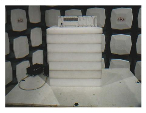
**Below 1 GHz Radiated Emission – Rear View**
