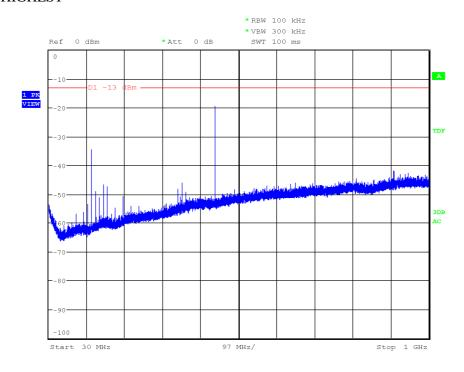
Note: The highest peak shown in the above plot is the carrier frequency.
