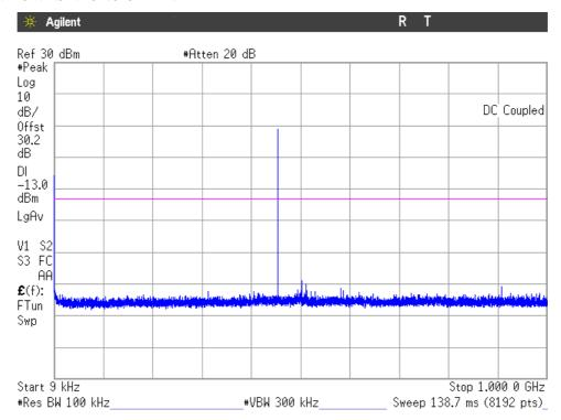
Note: The peak above the limit is the carrier frequency. The carrier was attenuated using a notch filter.
