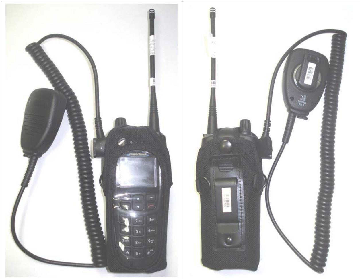
DUT with Nylon Case & Metal Belt-Clip Body-worn Accessory and Evolution Speaker-Microphone Audio Accessory
