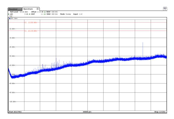
Note: The highest peak shown in the plot is the carrier frequency.
