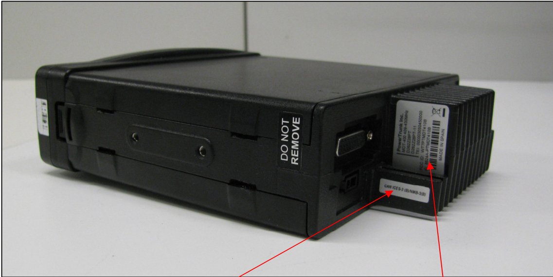
Model identification label 0000 PowerTrunk Inc. MDT-400 409-430 MHz D262228PT D262N28PT-11 TEI: 00000303xxxxxx0 FCC ID: W17PTMD1410B IC: 8624A-PTMD1410B MADE IN SPAIN
