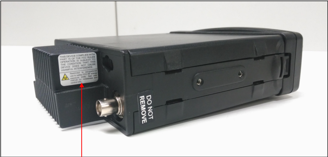
FCC Part 15 and RF Exposure compliance label THIS DEVICE COMPLIES WITH PART 15 OF THE FCC RULES. OPERATION IS SUBJECT TO THE CONDITION THAT THIS DEVICE DOES NOT CAUSE HARMFUL INTERFERENCE. Restricted to occupational use to satisfy FCC RF energy exposure limits. See user manual for awareness and control info.
