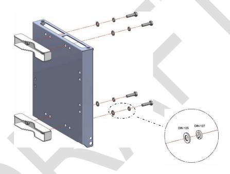
b) Install the bracket to the desired final location on the mast/pole. Embrace the 2 holes clamps and screw these to the bracket with a 17 mm wrench and 20 Nm torque. Due to the length of the bolts it is advisable to screw them slowly.
