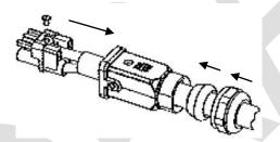
• Fix the assembly tightening the top locking screw and tightening the cable gland nut on the back of the hood/housing.
