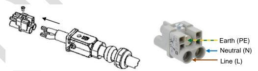
• Fix each wire tightening each pin from the front side with a hexagonal screwdriver (Allen number 2).
