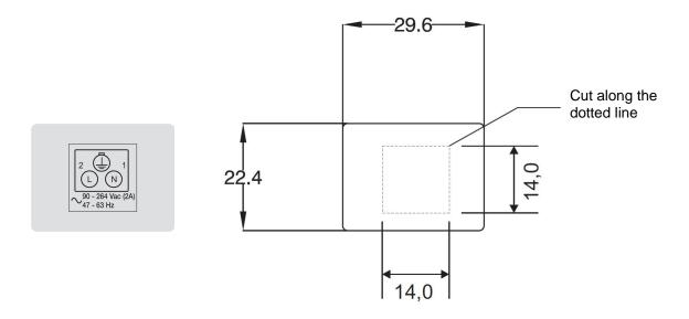
2.9 POWER SUPPLY IDENTIFICATION LABEL (MBS UNIT -K WITH VDC SUPPLY OPTION)
