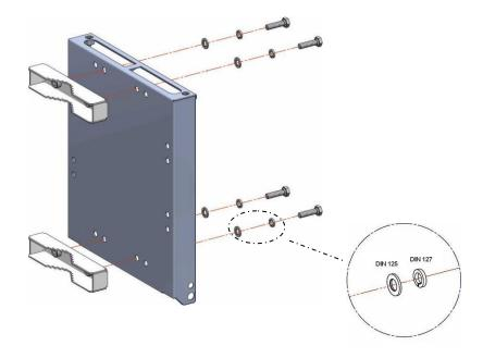
b) Install the bracket to the desired final location on the mast/pole. Embrace the 2 holes clamps and screw these to the bracket with a 0.67 in wrench and 20 Nm torque. Due to the length of the bolts it is advisable to screw them slowly.
