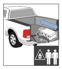
**Note:** the set composed by MBS Unit and the PBS Accessory has a heavy weight, the actions of loading and unloading into the vehicle must be done by at least two persons.
