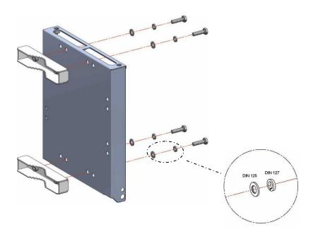
b) Install the bracket to the desired final location on the mast/pole. Embrace the 2 holes clamps and screw these to the bracket with a 0.67 in wrench and 20 Nm torque. Due to the length of the bolts it is advisable to screw them slowly.
