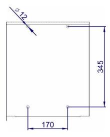
2. Drill holes on the wall and insert a rawlplug in each hole.
