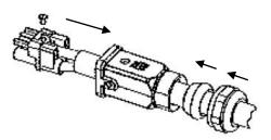
Fix the assembly tightening the top locking screw and tightening the cable gland nut on the back of the hood/housing.
