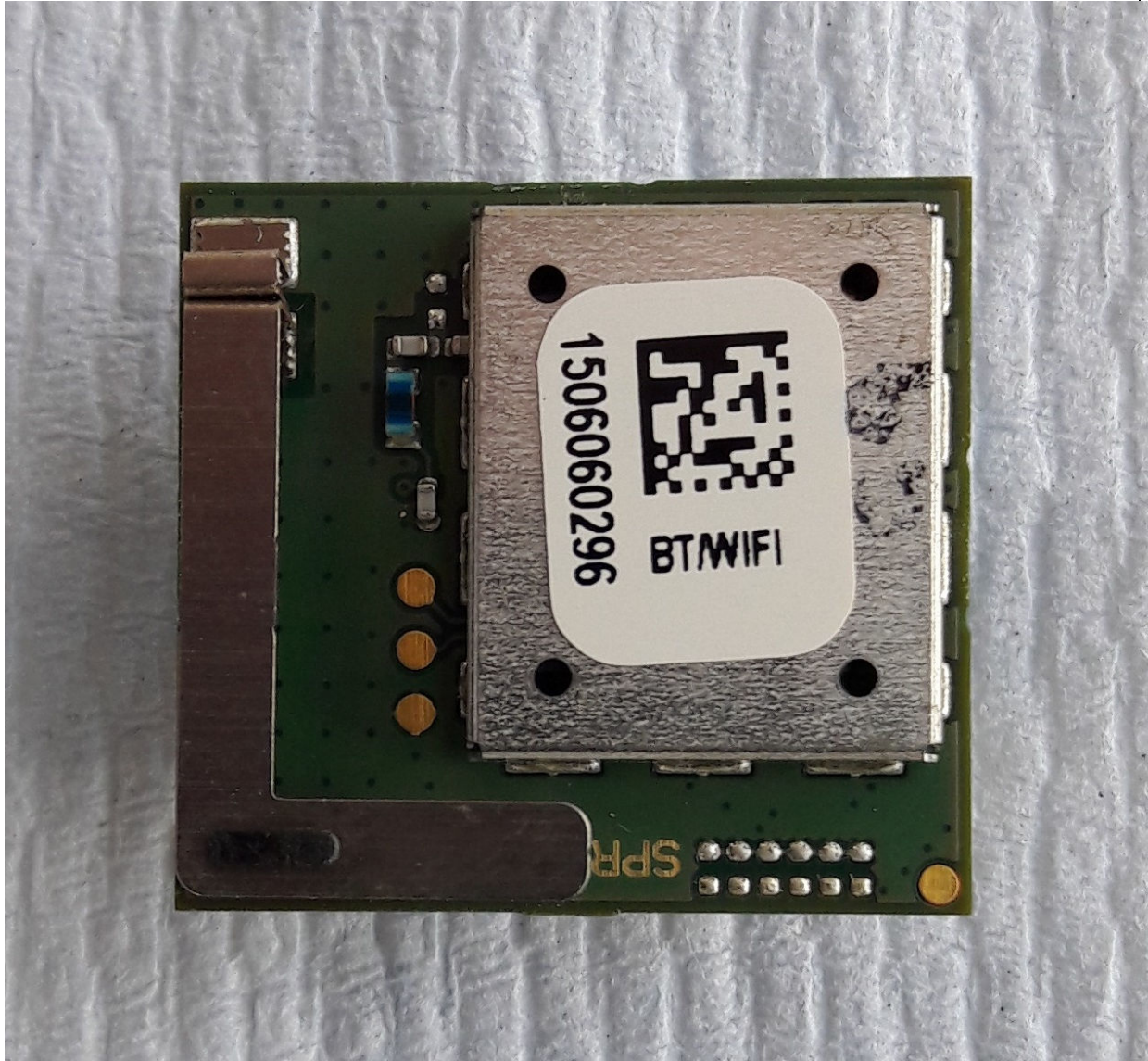
HTT-500-2 Bluetooth Module with screening can
