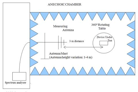
Shielded Control Room For Radiated Measurements
