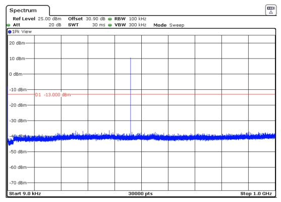
Note: The peak above the limit is the carrier frequency. The carrier was attenuated using a notch filter.
