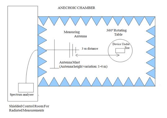
Radiated measurements above 1 GHz.
