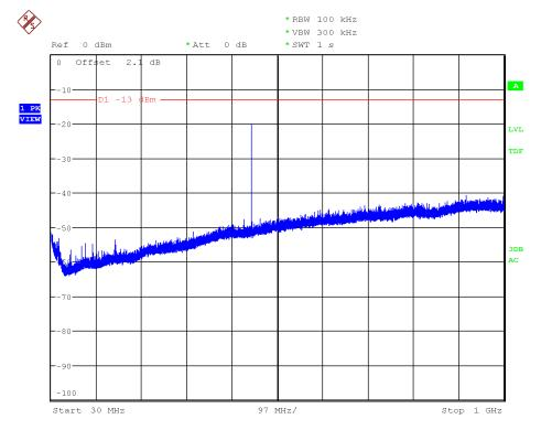
Note: The highest peak shown in the above plot is the carrier frequency.
