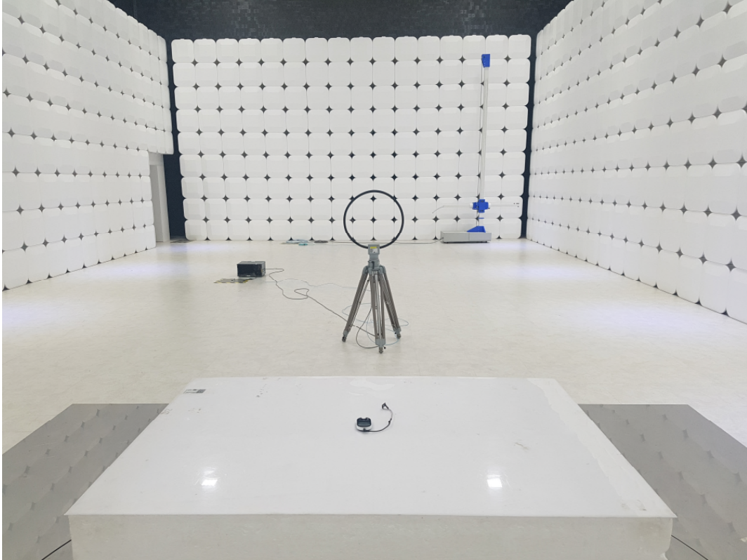
Radiated emission test (9 kHz to 30 MHz)
