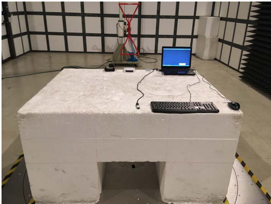
Radiated Emissions- Rear View (Below 1G)
