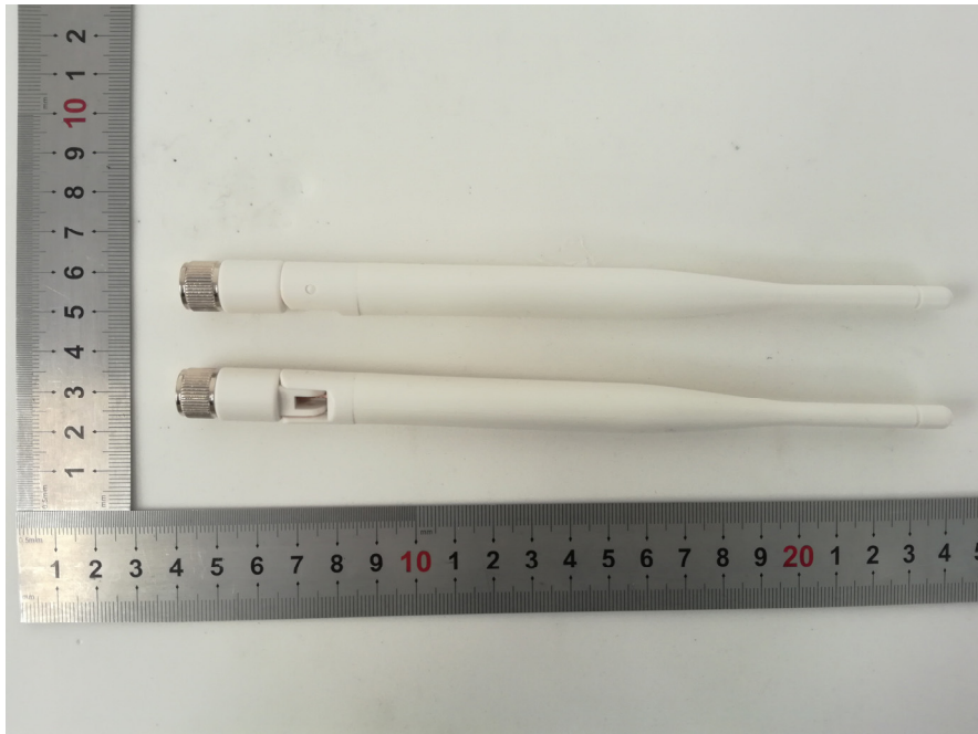
EUT – Antenna Connector Port View
