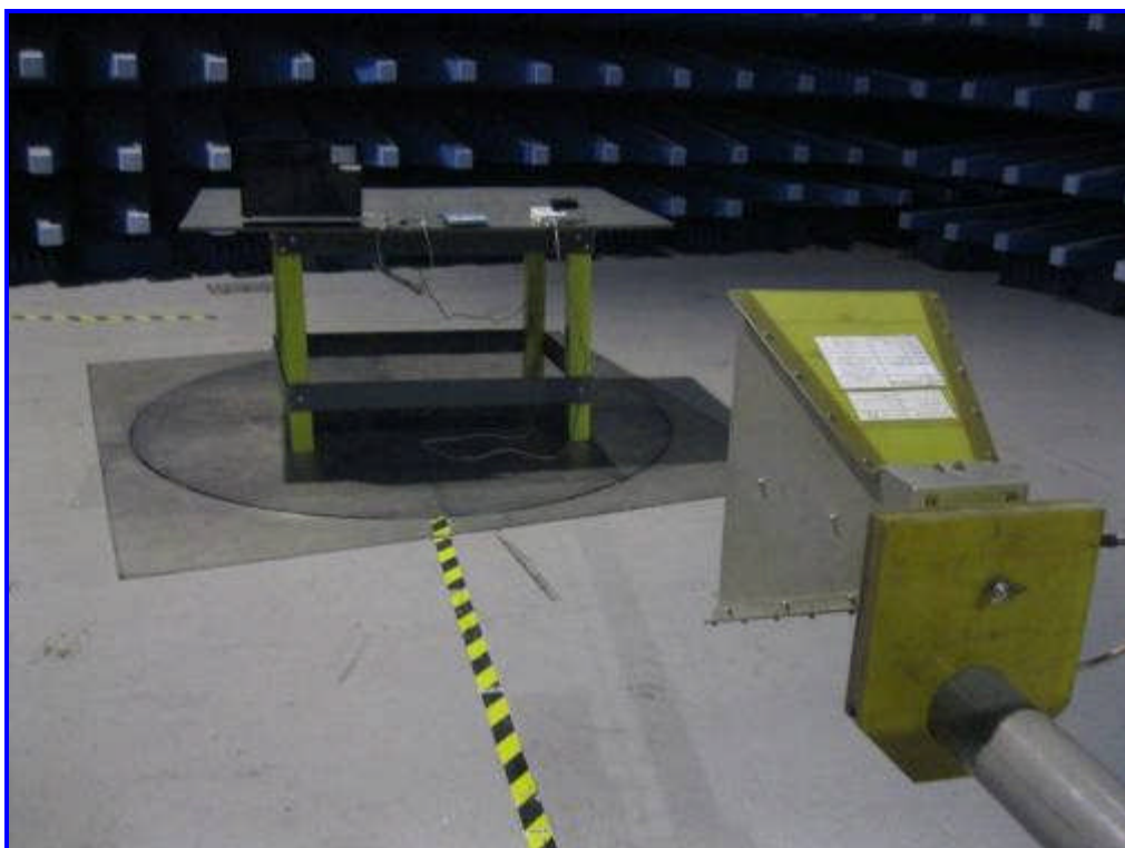
Radiated Emission Test Setup Front View above 1GHz
