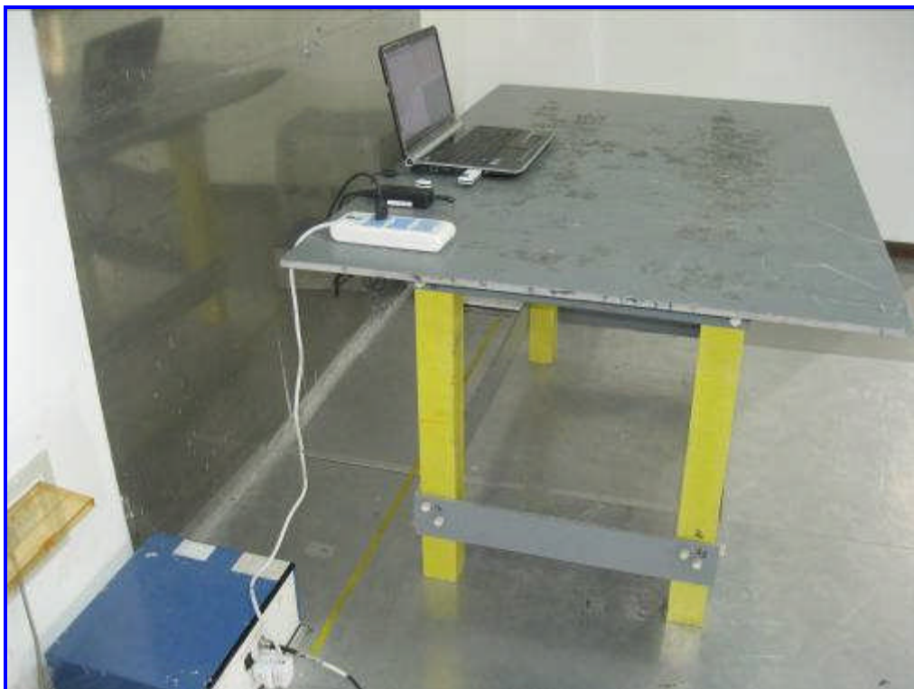
Conducted Emission Test Setup Side View
