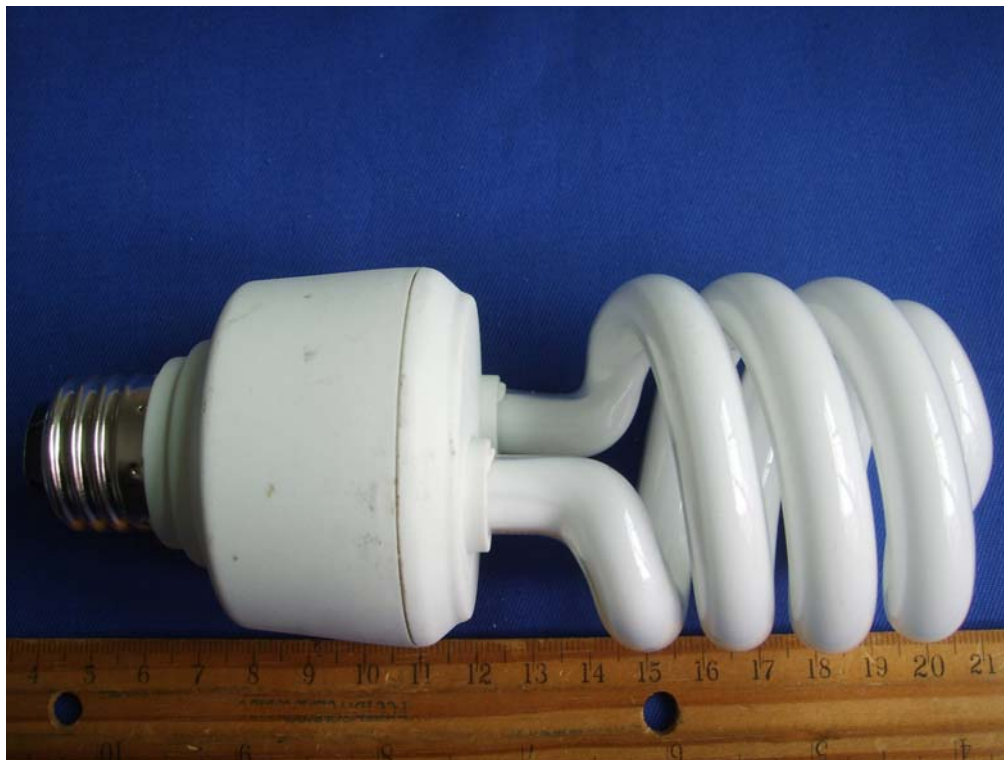
EUT - General View (HLT4S12/20/26W)
