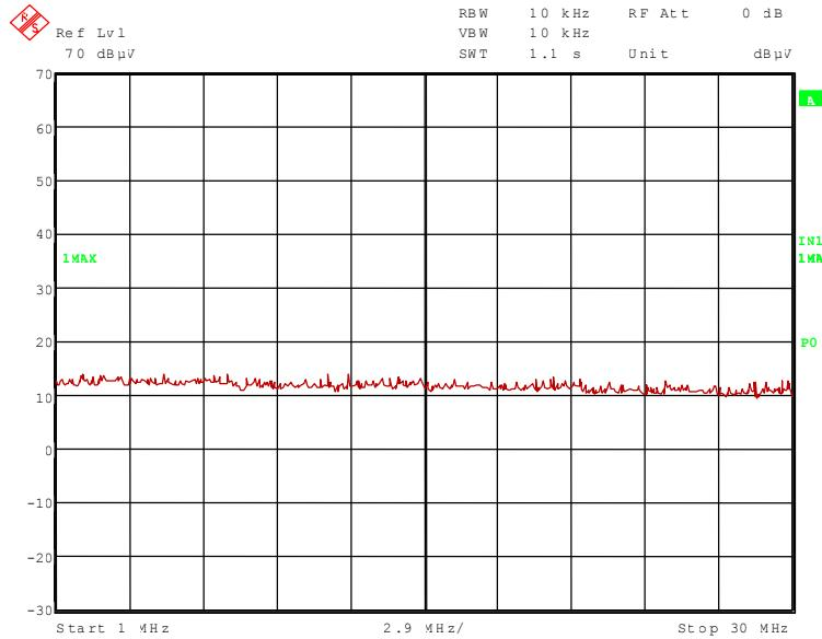
No significant emissions above the noise floor of the measuring system found in this frequency range, so no final measurement on the outdoor test site were carried out.
