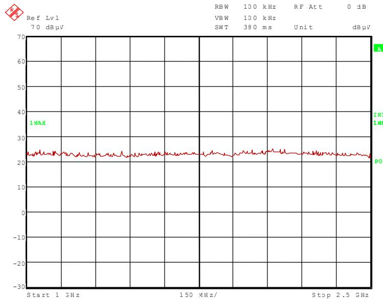
No significant emissions above the noise floor of the measuring system found in this frequency range, so no final measurements were carried out.
