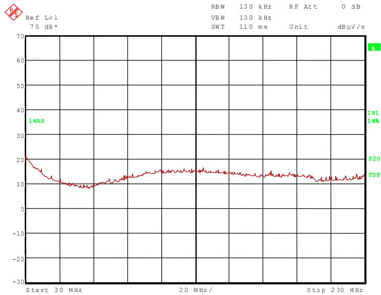
82373\_13.wmf: Spurious radiation from 230 MHz to 1 GHz:
