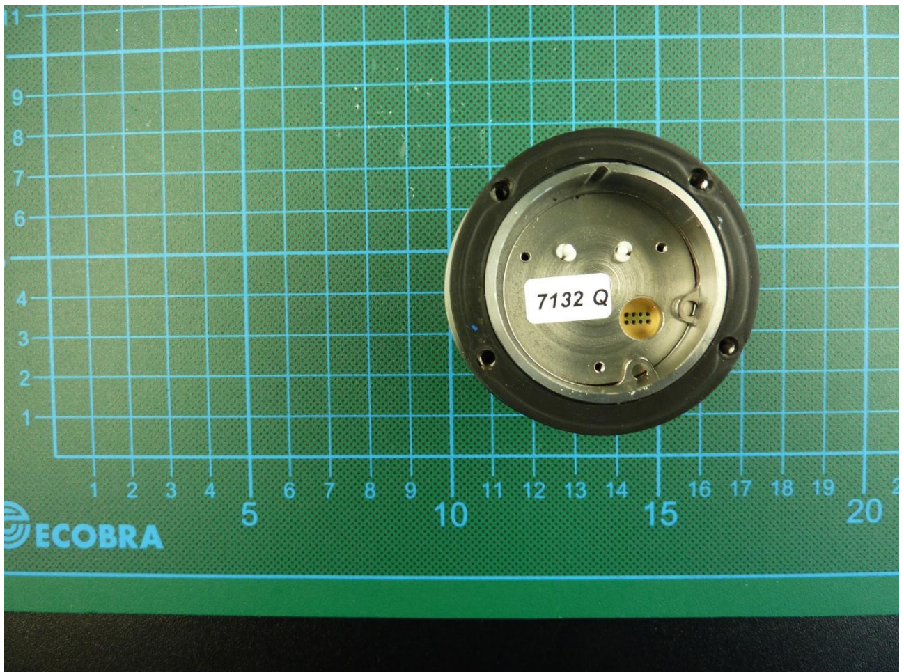
161191_18.jpg: EUT, PCB 1 removed
