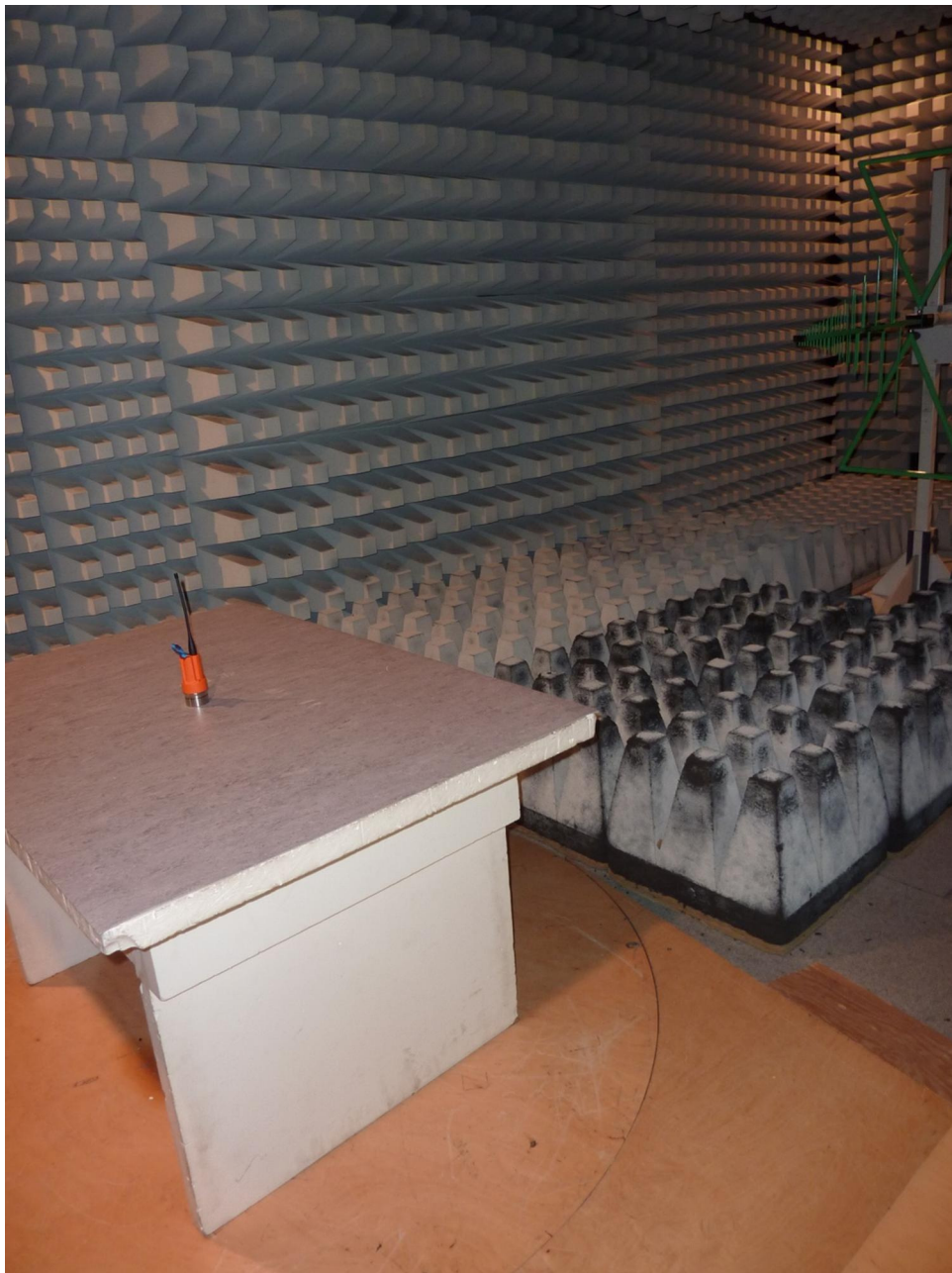
161191_02.JPG: Test setup - Radiated emission (fully anechoic chamber)
