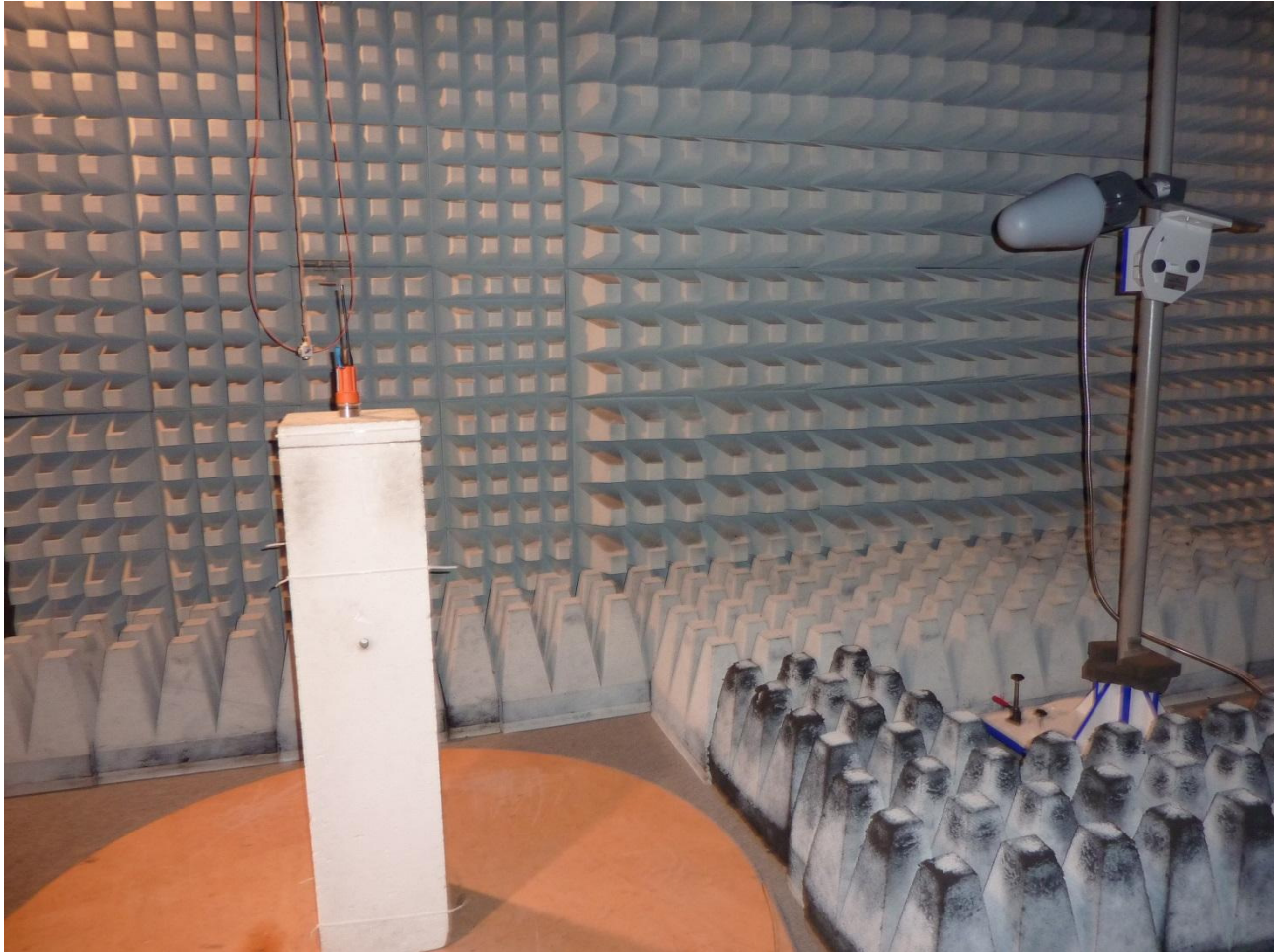
161191_03.JPG: Test setup - Radiated emission (fully anechoic chamber)
