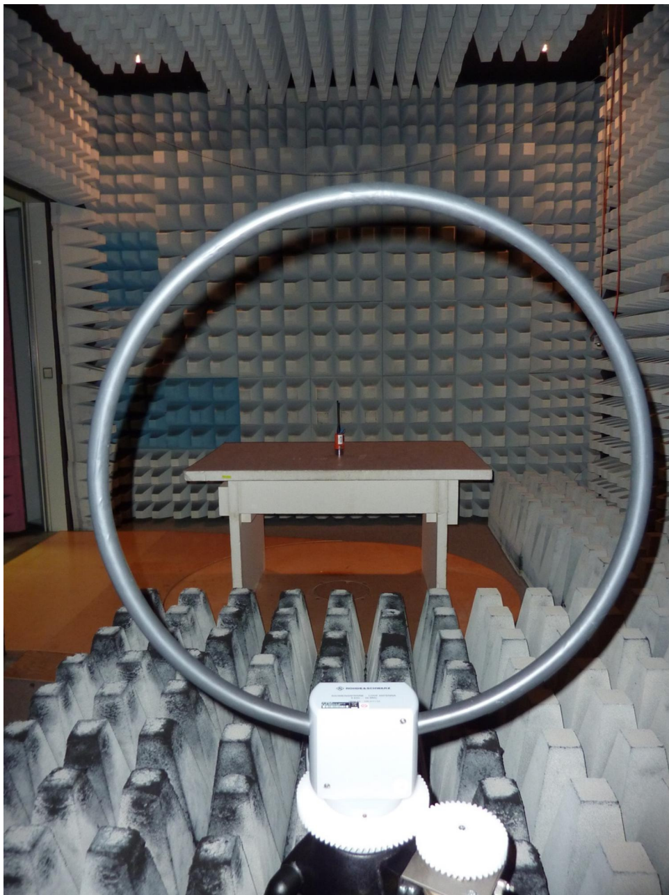
161191_01.JPG: Test setup - Radiated emission (fully anechoic chamber)
