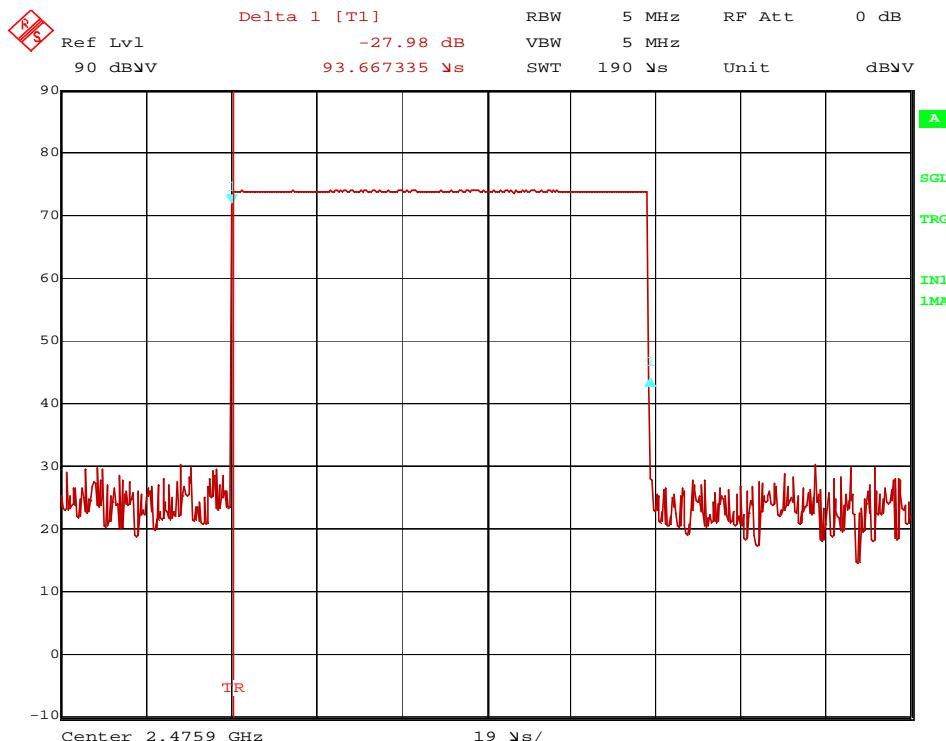
140852 Low DutyCycle M1: Duty cycle measurement 1 on channel 11:
