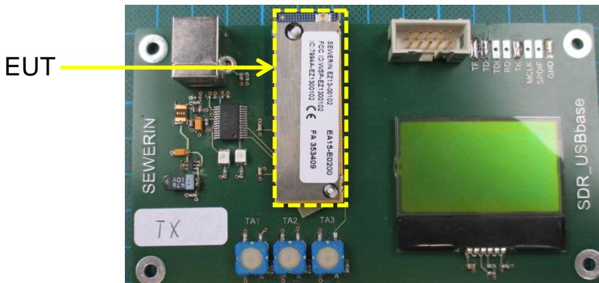
The EUT was powered with 5 V DC by an USB cable. The EUT was also connected to a Laptop computer using the same USB cable. The laptop contained special test software to set the EUT into the applicable test modes for the test.
