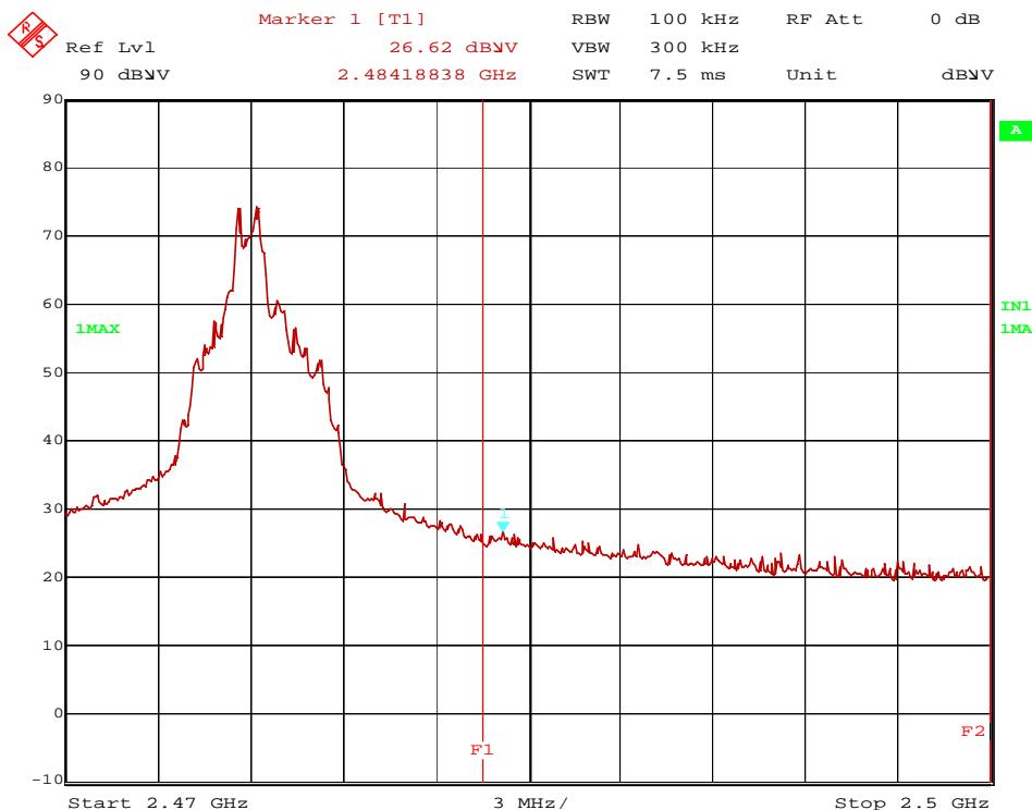
**Transmitter operates at the lower end of the assigned frequency band (operation mode 3)**
