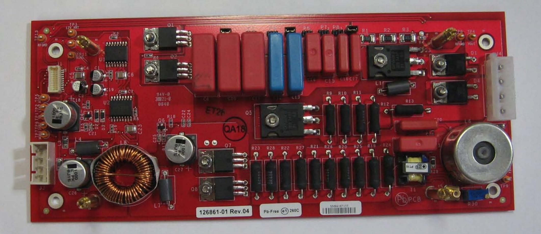
Driver board- lower PCB underside
