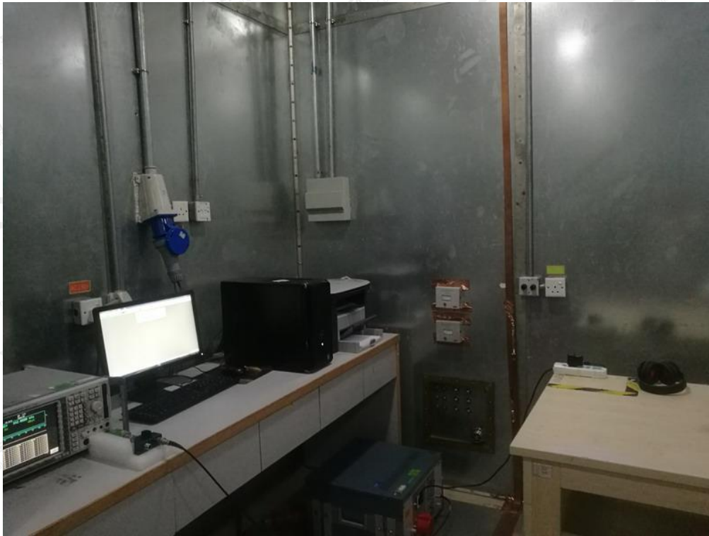
FCC RADIATED EMISSION TEST SETUP
