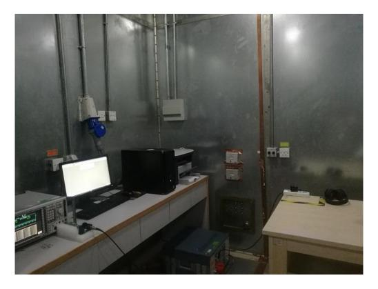
FCC RADIATED EMISSION TEST SETUP
