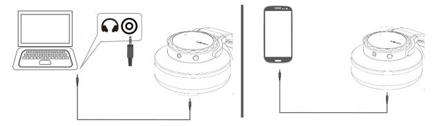
\*Notice: 1. When plug in the aux hole, the headphone button is no function
