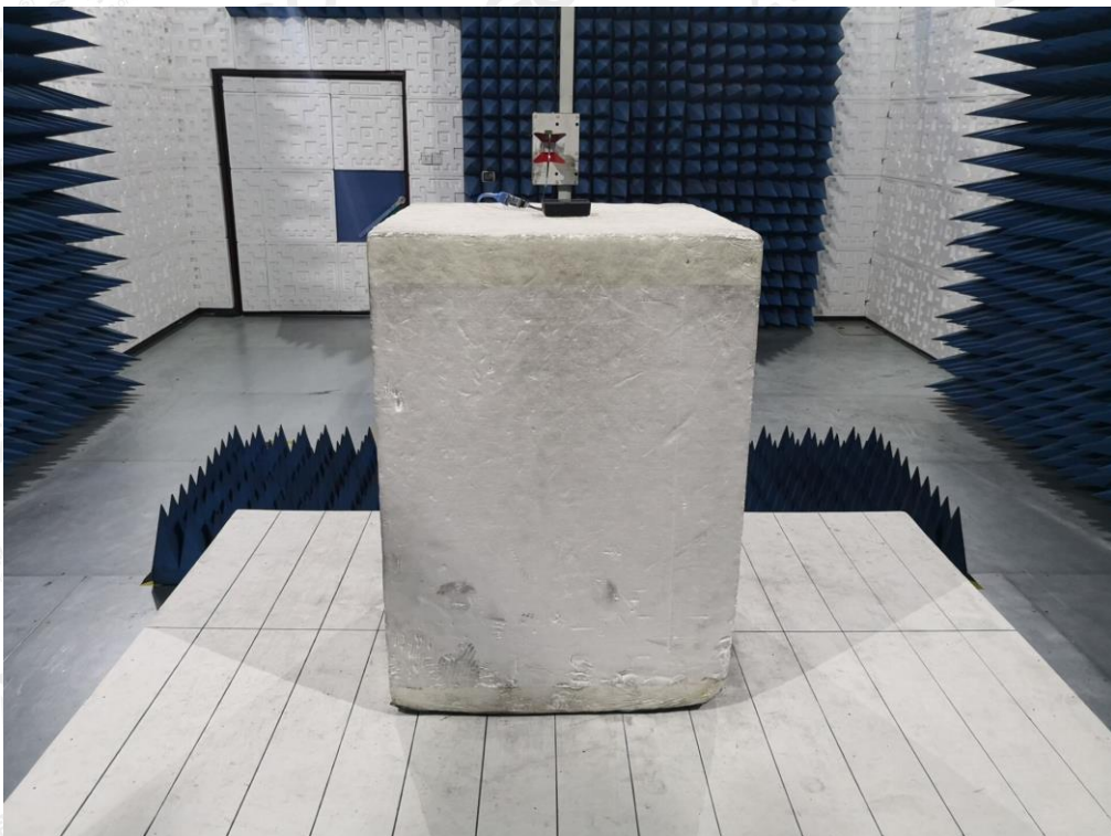
RADIATED EMISSION TEST SETUP ABOVE 1GHZ
