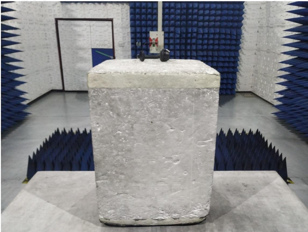
RADIATED EMISSION TEST SETUP ABOVE 1GHZ
