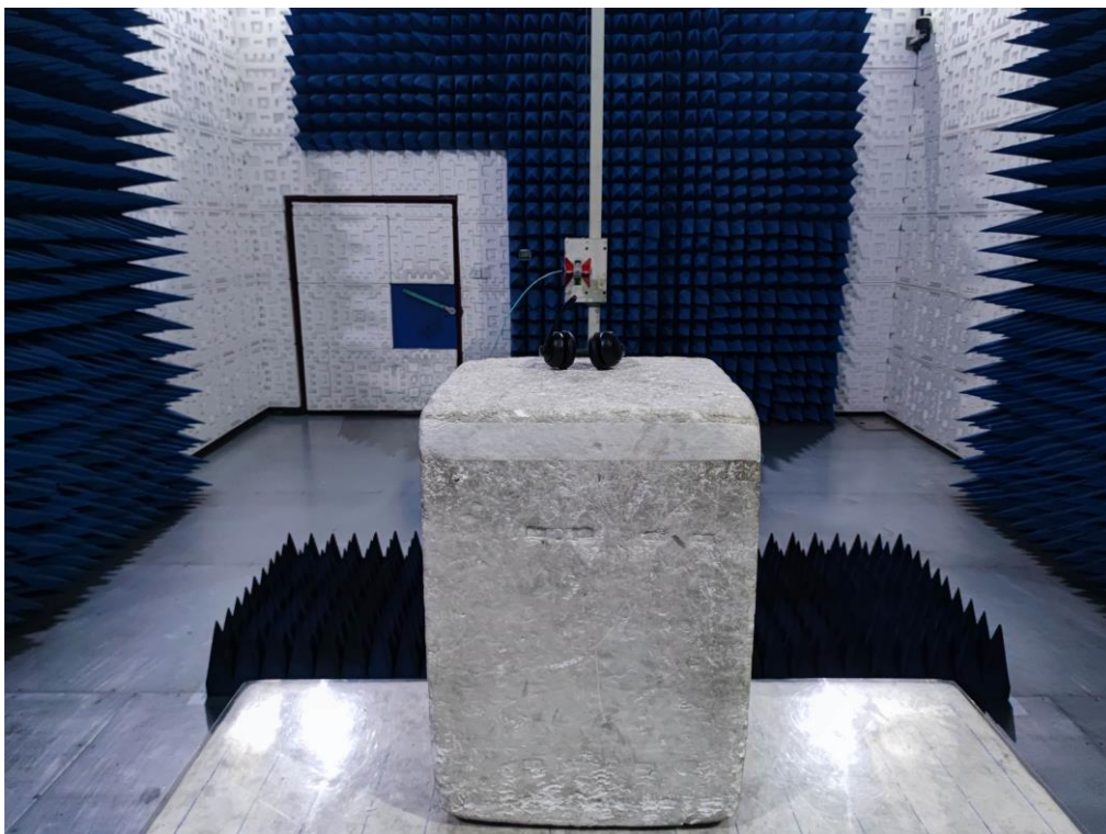
RADIATED EMISSION TEST SETUP ABOVE 1GHz
