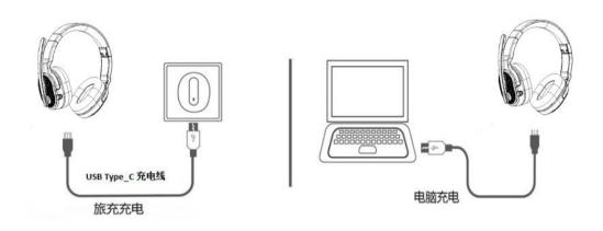
Charging port, USB head connected to USB charger (car charge, travel charge, computer USB, etc.)
