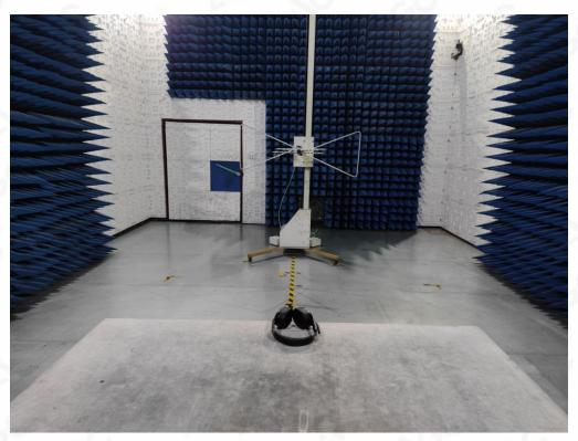
RADIATED EMISSION TEST SETUP ABOVE 1GHz
