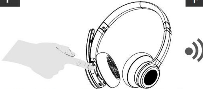
In the off state, switch on the device. When there is no pairing record, it will automatically enter the pairing mode, and the LED flashes red and blue alternately. The pairing state prompt sound "Pairing".
