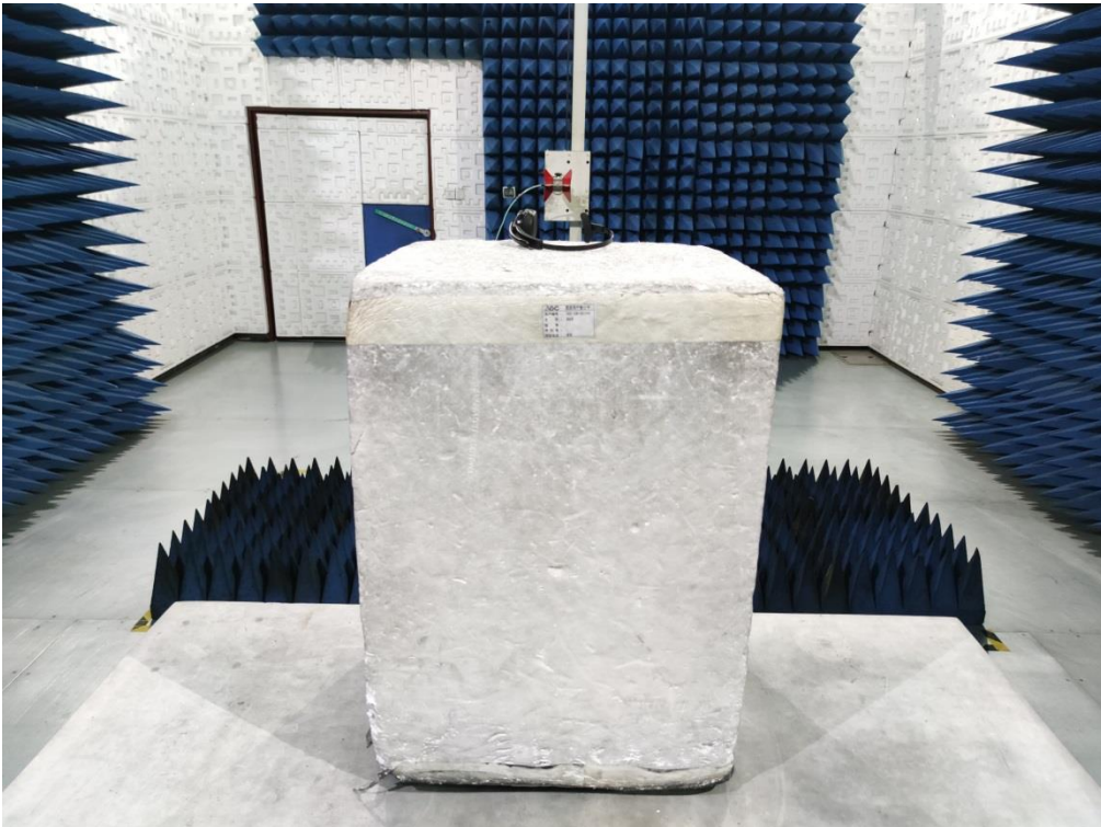
RADIATED EMISSION TEST SETUP ABOVE 1GHz
