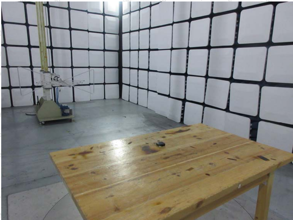
Photo of Radiation Emission Test
