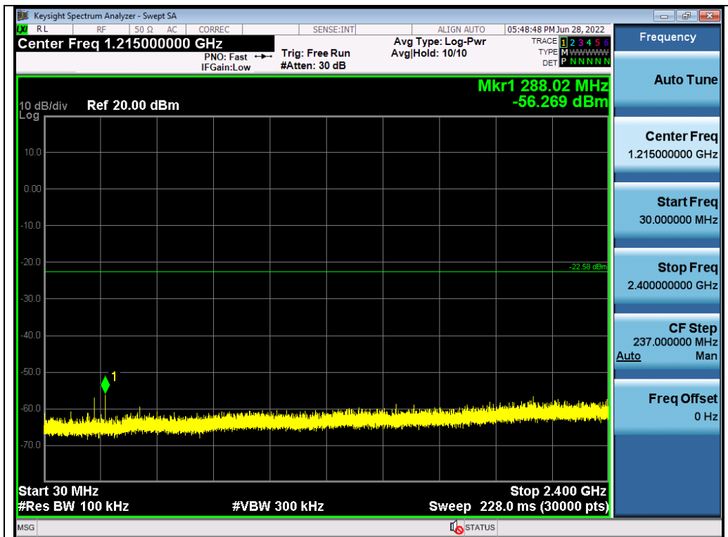
Test_Graph_EDR_ANT1_2480_2Mbps_Lower Band Emissions
